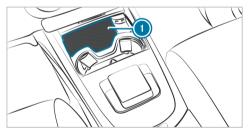
Place the mobile phone as close as possible to the center of mat () with the display facing up.
