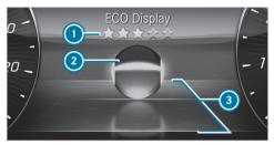
The ECO display shows an evaluation of your driving style on the driver display depending on the situation. This enables you to check the efficiency of your driving style and adjust it if necessary. The ECO Display menu shows a ball (2) that will roll forwards or backwards in the direction of travel on a stylized road according to the driving characteristics.
