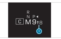
When gearshift recommendation () appears on the driver's display, shift to the recommended gear.
