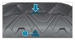
Six marks ① show where the bar indicators (arrow) are integrated into the tire tread. They are
