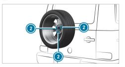
Removing the wheel from the spare wheel carrier and attaching the defective wheel
