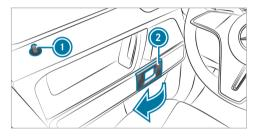
To unlock and open a front door: pull door handle 2.
