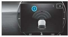
If autonomous braking, situation-related based assistance or evasive action has occurred, pop-up appears on the driver display. It automatically disappears after a short time.
