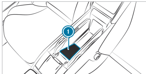
Charging mat in the stowage compartment of the rear passenger compartment center console
